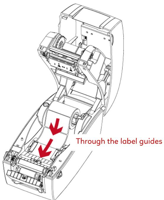
3. Pull the label liner through the platen and the steel of the label dispenser.
