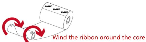
3. A ribbon module is assembled as below.
