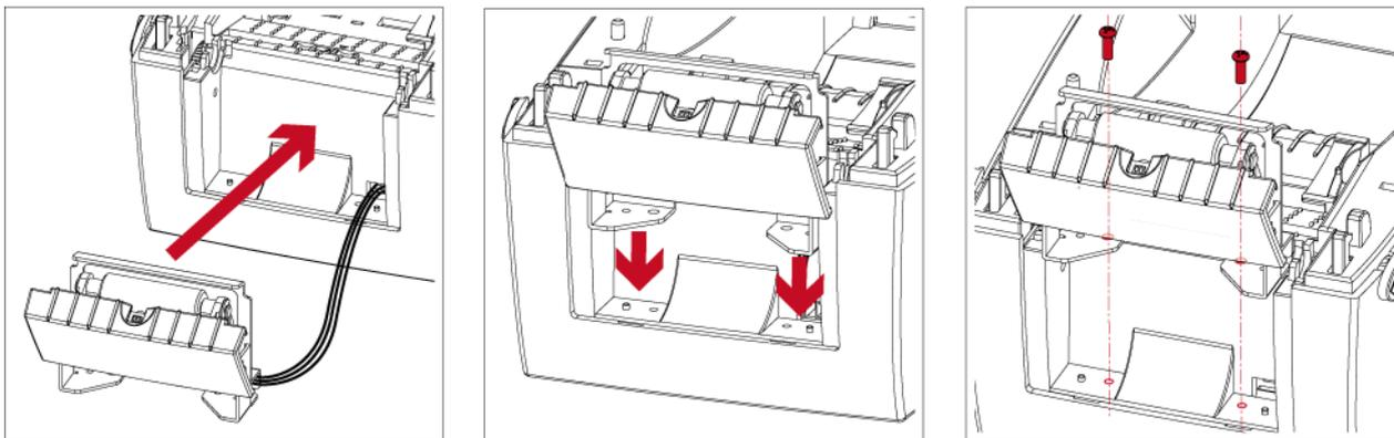
3. Place the platen back to the printer and lock the clips.
