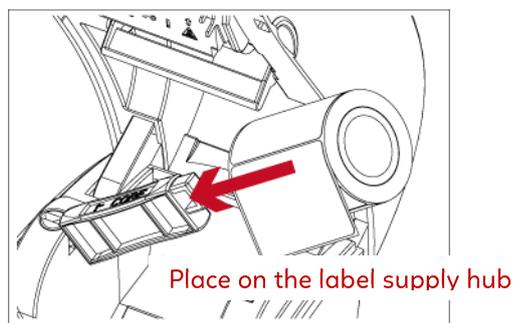
3. Push the label supply module downward and close the release catch.
