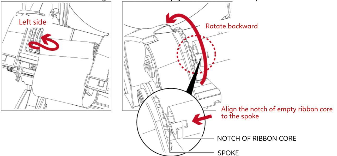
4. Turn the ribbon rewind wheel to tighten the ribbon until it has no wrinkles.
