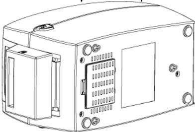
6. Open the cover on the bottom of printer.
