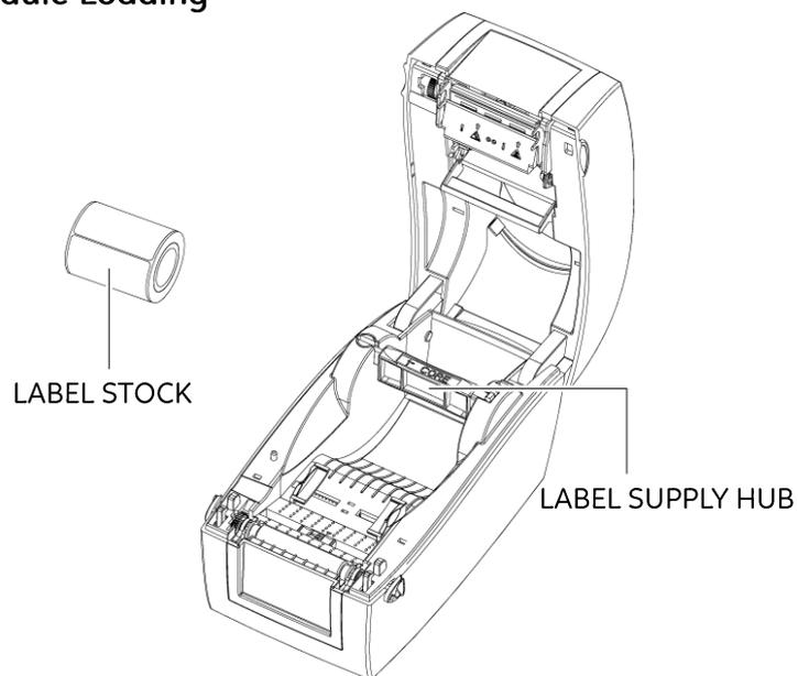
1. Unlock the release catch to lift the label supply hub.
