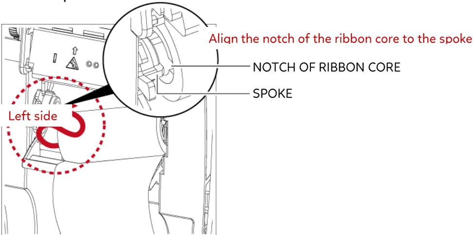
3. The ribbon supply module loading is completed.
