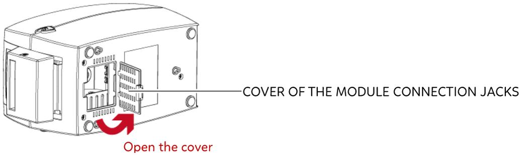
7. Plug the connector for the cutter to the jack.
