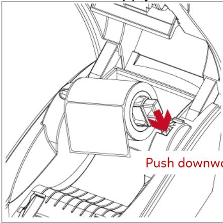
4. A new label supply module is completed.
