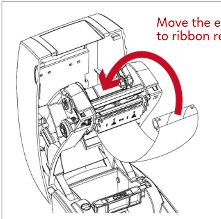
Move the empty ribbon core upward
