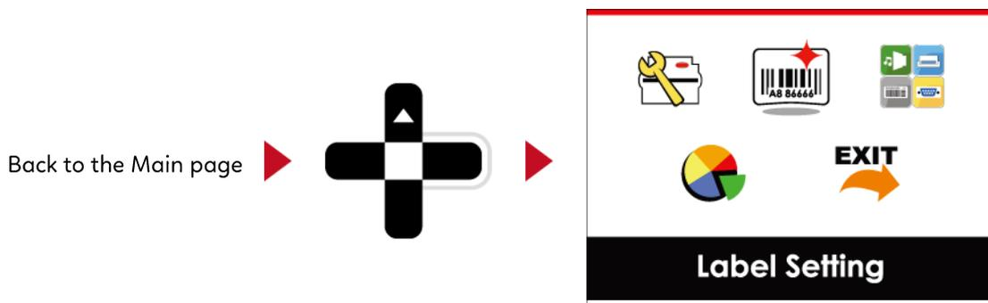
On MAIN PAGE, select the “EXIT” icon and press the FEED button to exit from SETTING MODE and the printer goes back to READY status.
